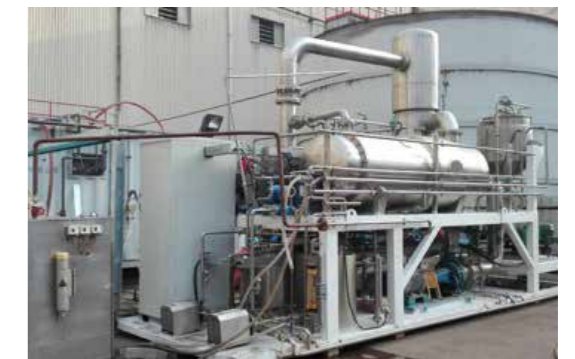
浓盐水结晶分盐技术实验平台 RESEARCH & EXPERIMENT PLATFORM FOR CONCENTRATE CRYSTALLIZATION AND SALT PURIFICATION TECHNOLOGY
